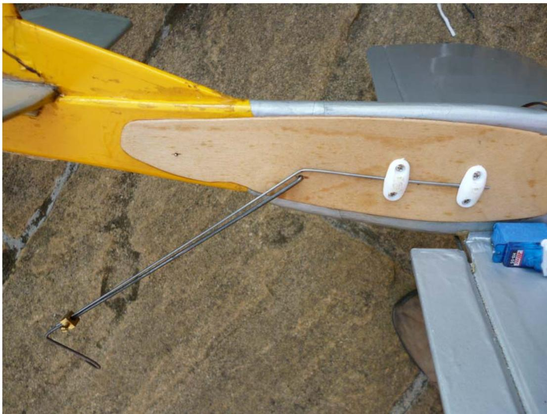
Arrester wire, adjustable torsion bar and throttle servo.
