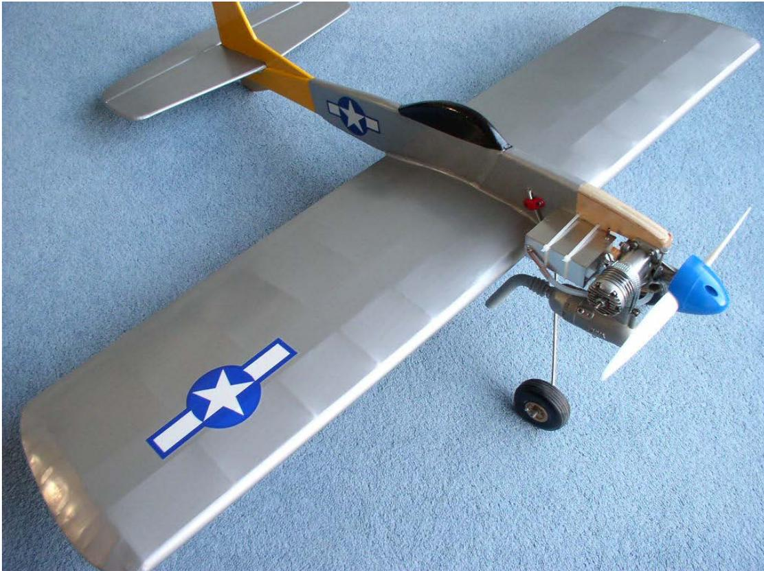
36" span profile model before conversion to basic carrier deck specification.
