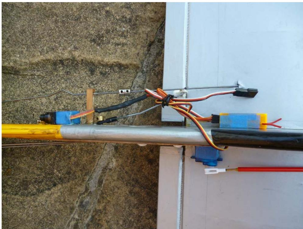
Top view showing arrester release servo, flap fixing, throttle servo and receiver.
